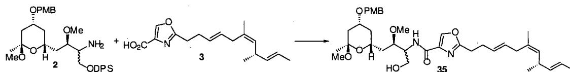
To a stirred solution of the carboxylic acid **3** (14 mg, 0.048 mmol) and the amine **2** (32 mg, 0.052 mmol) in DMF (0.3 ml) at 0 °C was successively added dropwise DEPC (0.010 ml, 0.061 mmol) and triethylamine (0.014 ml, 0.101 mmol). After being stirred at 0 °C for 2 h and then at room temperature for 7.5 h, the reaction mixture was diluted
